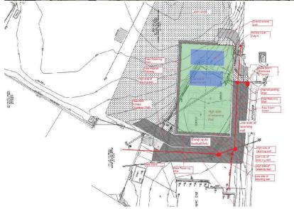
Install retaining walls, new storm manholes and sewer, stairs, and handicap accessible path/driveway to upper field.
